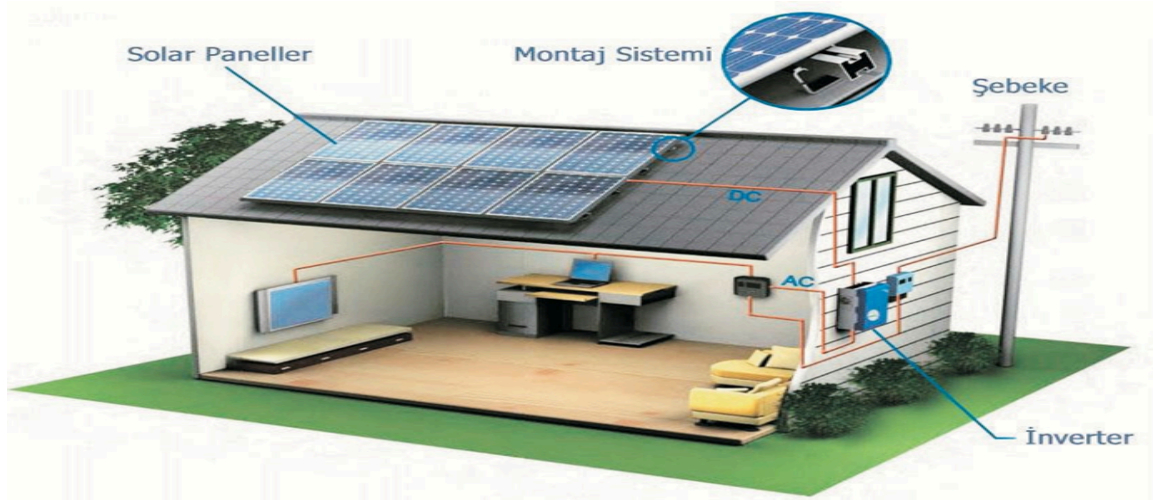
Picture: 1.5: Photovoltaic solar system
