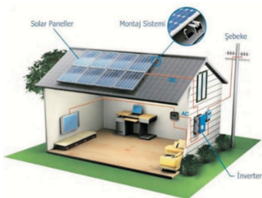
Picture: 2.1: Photovoltaic solar system (on grid)
