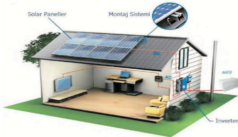
Picture: 2.2: Photovoltaic solar system (on grid)
