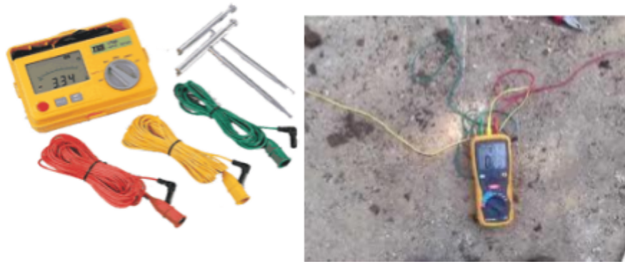
Resim 1.5: Megger measuring instrument
