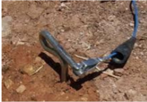
Photo 1.6: Meger pile connection and resistance measurement
