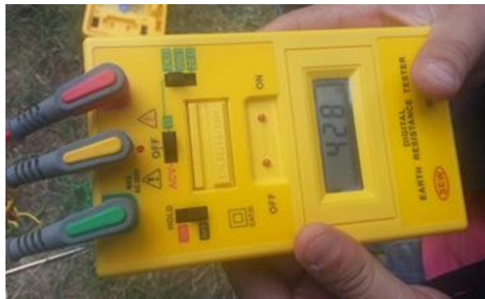
Picture 3.1: Digital grounding resistance measurement device
