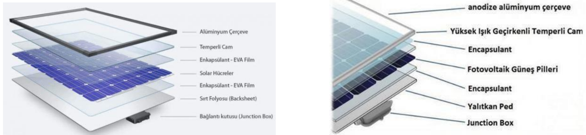
Picture 2.1: Structure of the solar panel
