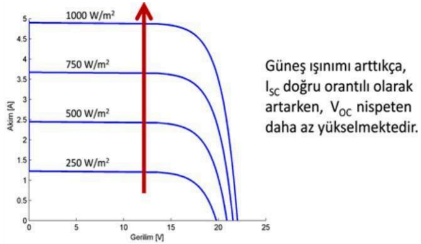
Figure 2.2: Change of current and voltage depending on solar radiation
