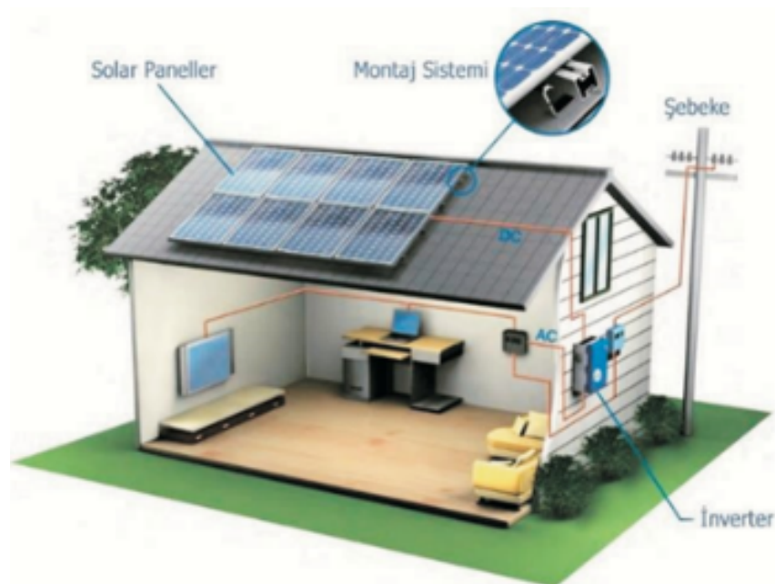
Picture: 2.1: Photovoltaic solar system (on grid)
