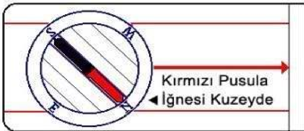
Figure 4.3: Turning until the north of the compass needle coincides with the north inside the compass slot
